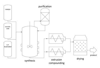
modelling the reaction process in MATLAB by using kinetic data from scientific literature. Therefore, it is now possible to monitor the amount of reactants and product at every timestep during the reaction, as well as the reaction volume and the required heating energy for the reaction to run properly. A simplified process flow schem is depicted here.
