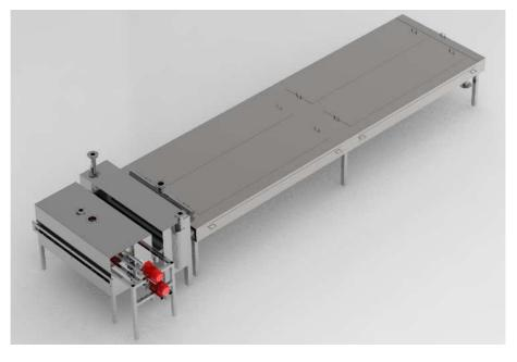
two outlet tubes at the bottom end of the chamber. The foil is transported over small rolls, which ensure that as little friction as possible is applied to it. Easy access for maintenance is given by opening the covers of the dryer. Stainless steel has been chosen as material to prevent corrosion for every part that comes into direct contact with the solvent-containing adhesive or the solvent-containing nitrogen. The transport rolls inside the dryer consist of
