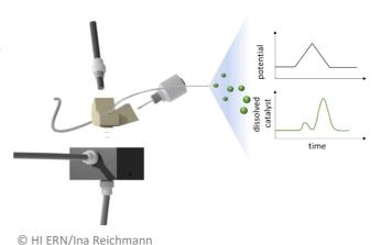
(ICP-MS) setups. The focus is on investigating, understanding, and mitigating the catalyst's corrosion processes.
