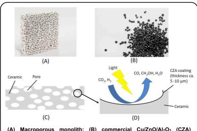
(A) Macroporous monolith; (B) commercial Cu/ZnO/Al<sub>2</sub>O<sub>3</sub> (CZA) methanol synthesis catalyst; (C, D) Scheme of the monolith, the CZA coating and the photothermal conversion of CO<sub>2</sub> to methanol reaction.
