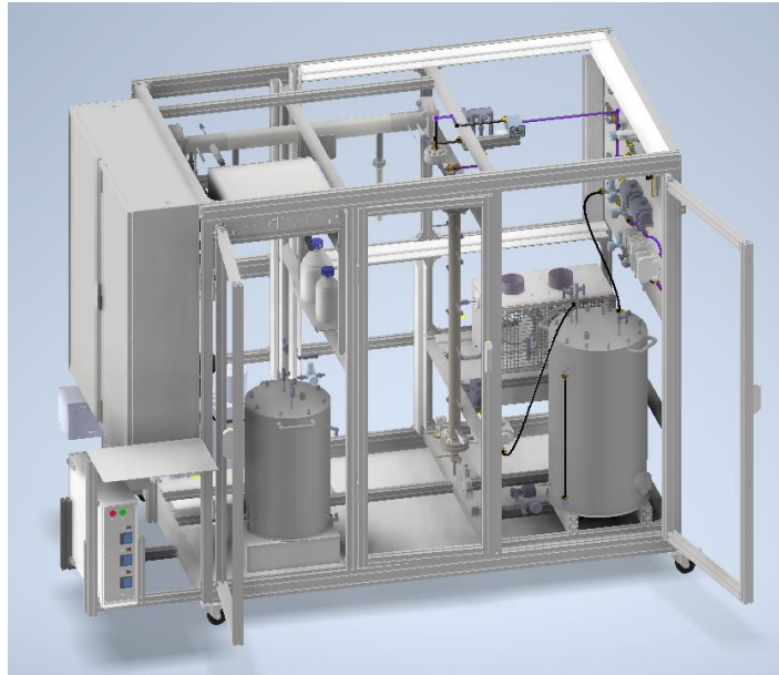
Fig. 2: 3D-Drawing of Plant for Oxidation of LOHCs
